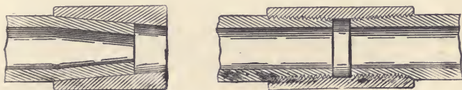
FIG. 114.—MAKING LEAD-PIPE JOINTS.
